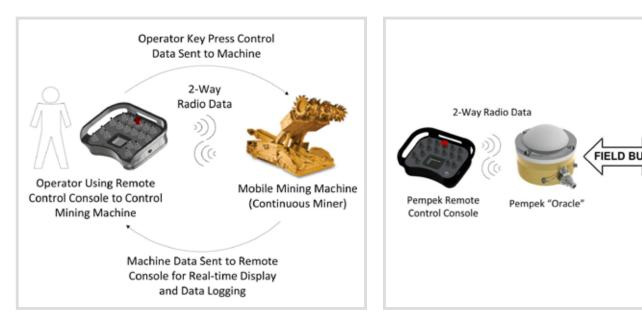
The remote console establishes and maintains a 2-way radio data link with the control system on-board the mobile mining machine. By way of this link, any keypress commands made by the operator are sent to the machine for control purposes.
