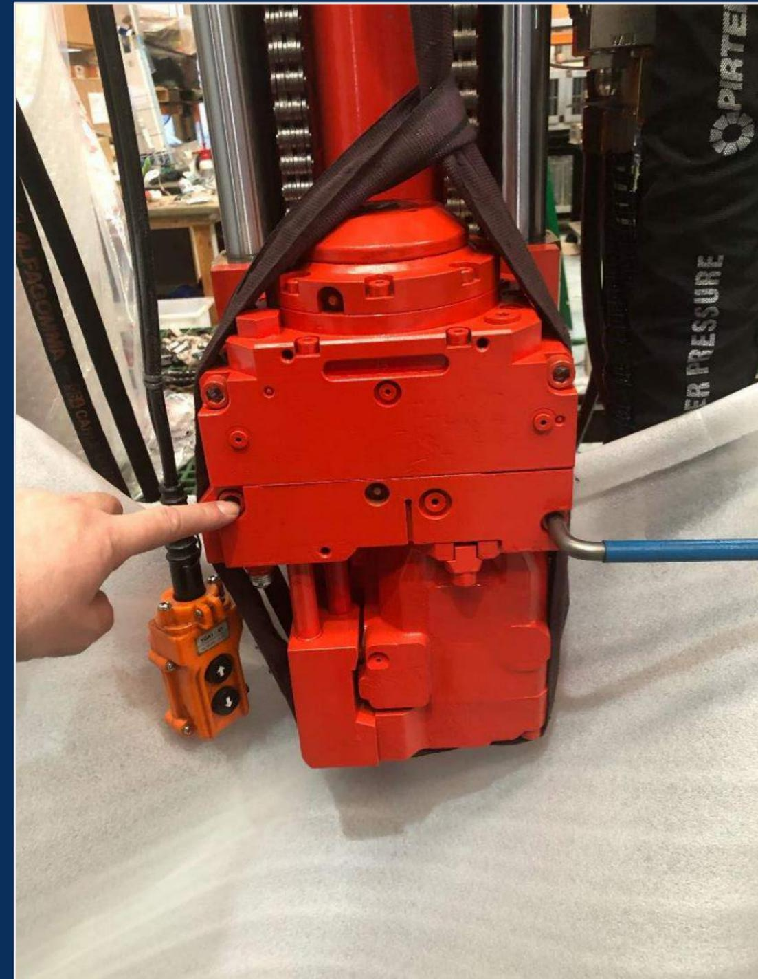
3. Balance lift sling and remove four cap screws
