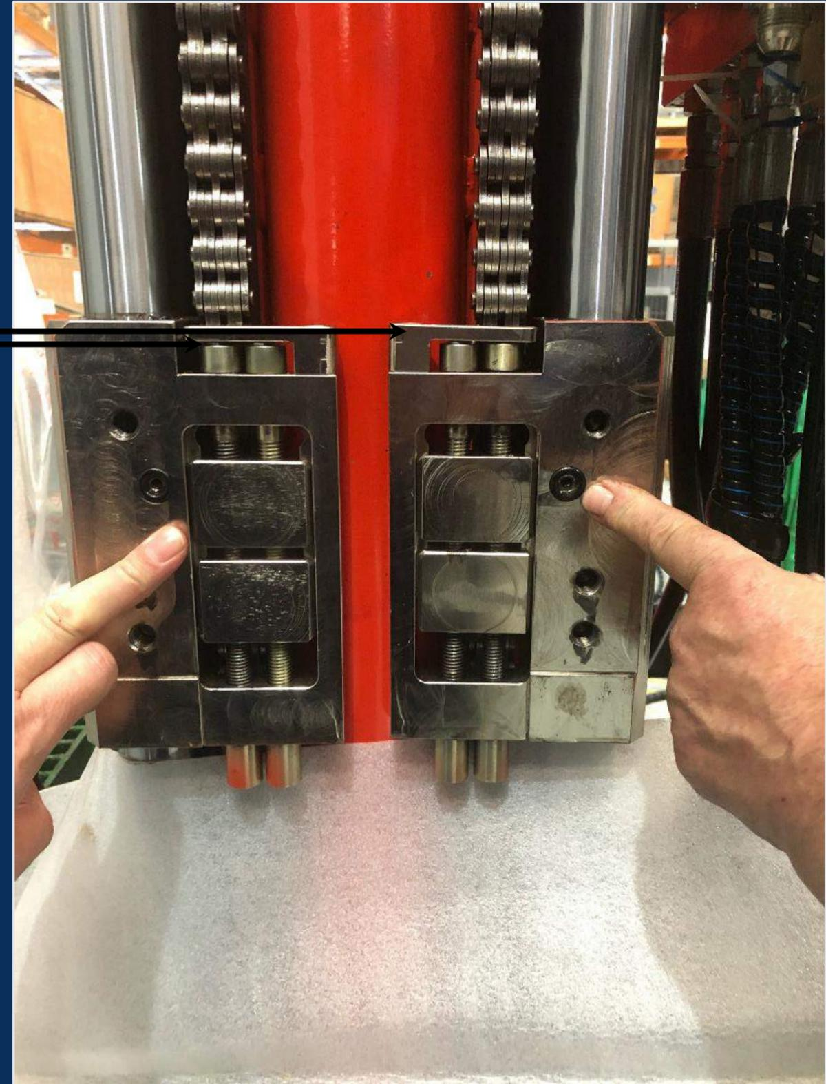
9. Check O rings installed, reinstall mount plate + check O rings
