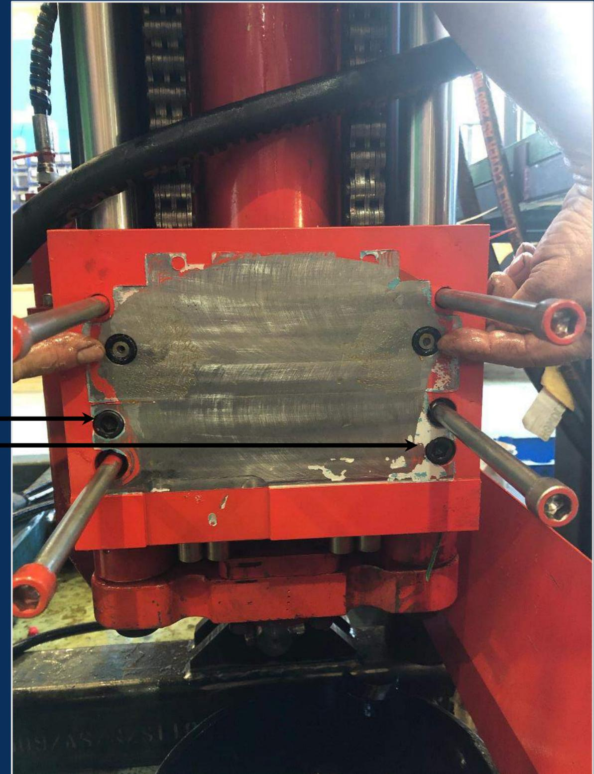
13. Adjust top and bottom tensioner screws X 2
