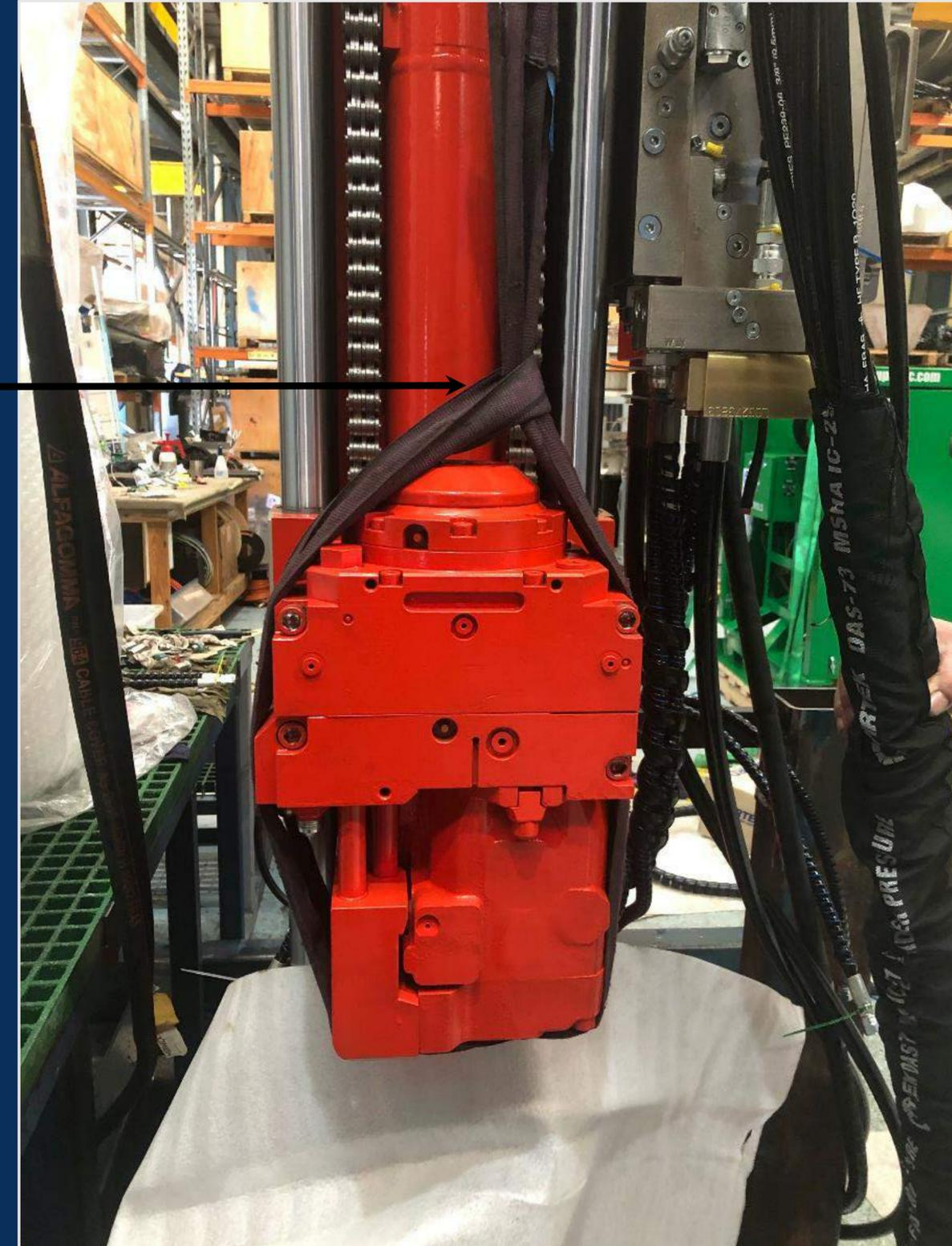
12. Remove 4 x Motor cap screws
