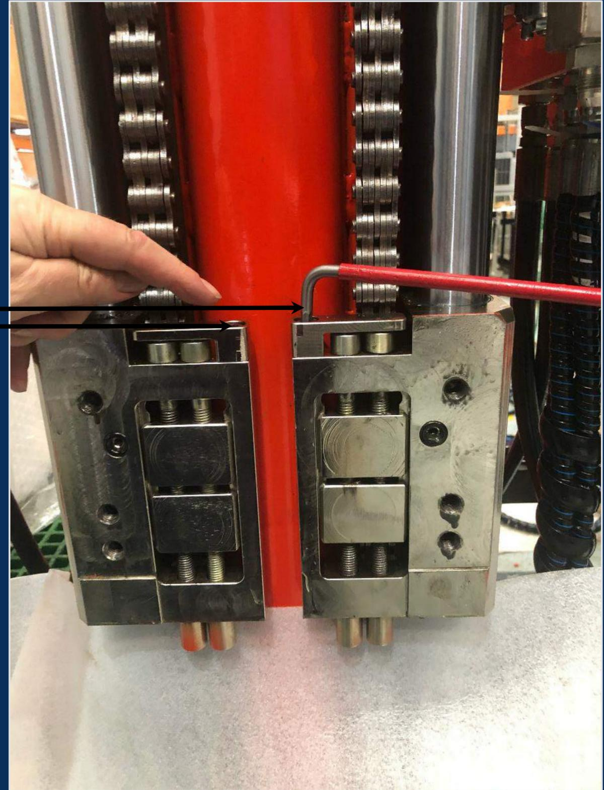
6. Adjust top and bottom tensioner screws X 2
