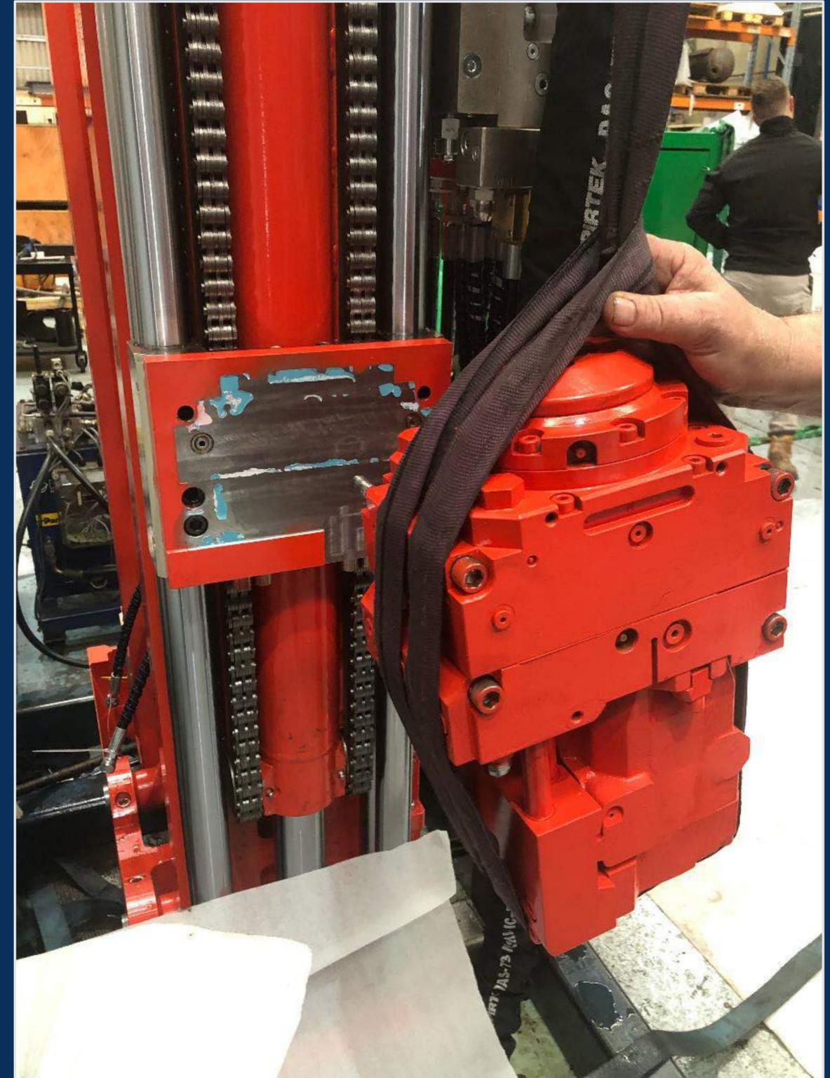
4. Remove 2 cap screws from motor plate.
