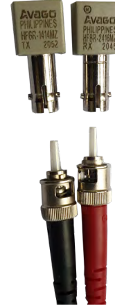
Image above Fibre Optic Patch ST-ST Multi-Mode
