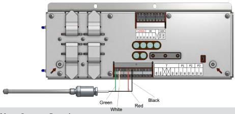
HBox 5 | Internal Wiring - Pressure Transducers
