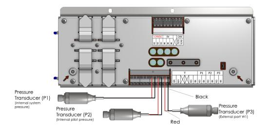
HBox 5 | Internal Wiring - CAN ID and Diagnostic Cable
