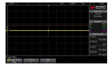
The PEMPEK L11V filter successfully mitigates the noise on motor drive pilot line and the PEMPEK L11V Filter earth switching mechanism decreases the touch potential from a dangerous 170V to a safe 35V.
